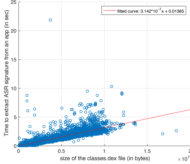
Figure 8: Time required to extract ASR signatures from an app, depending on the size of the classes.dex file.
